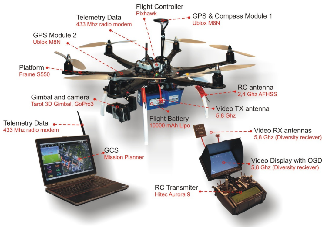
Fig. 2. Hexacopter platform hardware configuration and components assembly
