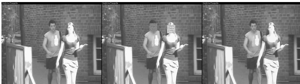
Figure 10: Real life example of the reversible anonymization: original frame (left), anonymized frame (center), de-anonymized frame (right)
