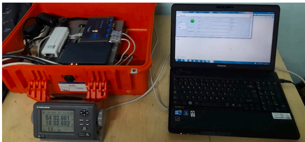
Fig. 9. Real-time satellite navigation data recording system.
