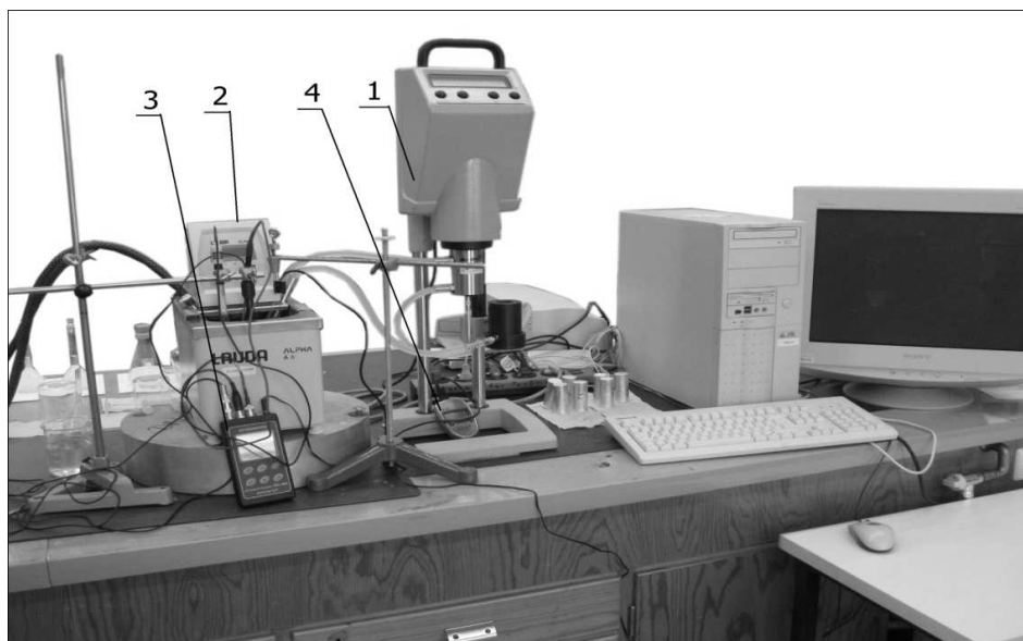
Figure 1: View of the experimental apparatus: 1 – viscometer, 2 – thermostat, 3 – pH and electrical conductivity meter, 4 – thermal conductivity meter.
