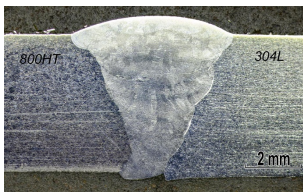
Figure 6. Cross-section of the Incoloy 800HT nickel alloy–304L austenitic stainless steel welded joint.
