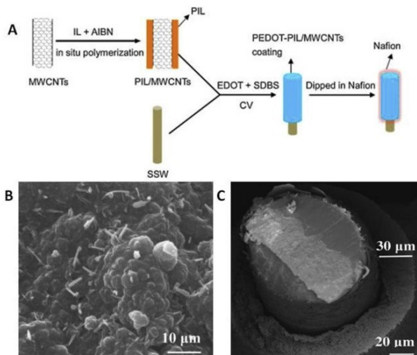
Fig. 6. The example of multi-component IL-based SPME fiber: a) steps of fiber fabrication; b) surface SEM image of the fiber of nodular accumulating structure with scattered MWCNTs; c) cross-section SEM image of the fiber [107] (Copyright 2016 by Elsevier).
