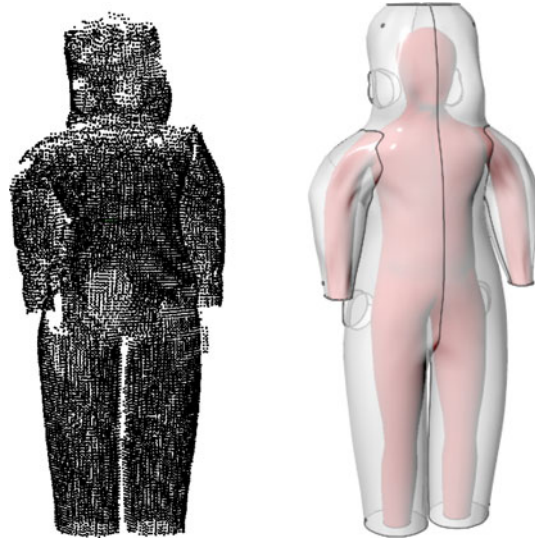
Fig. 4 Cloud points ( left ) and the reconstructed geometry ( right )
