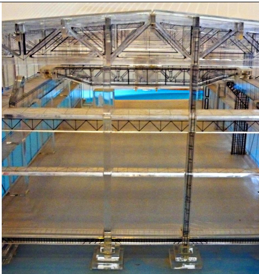
Figure 7: The model of an industrial hall with a crane showing the gable wall view
