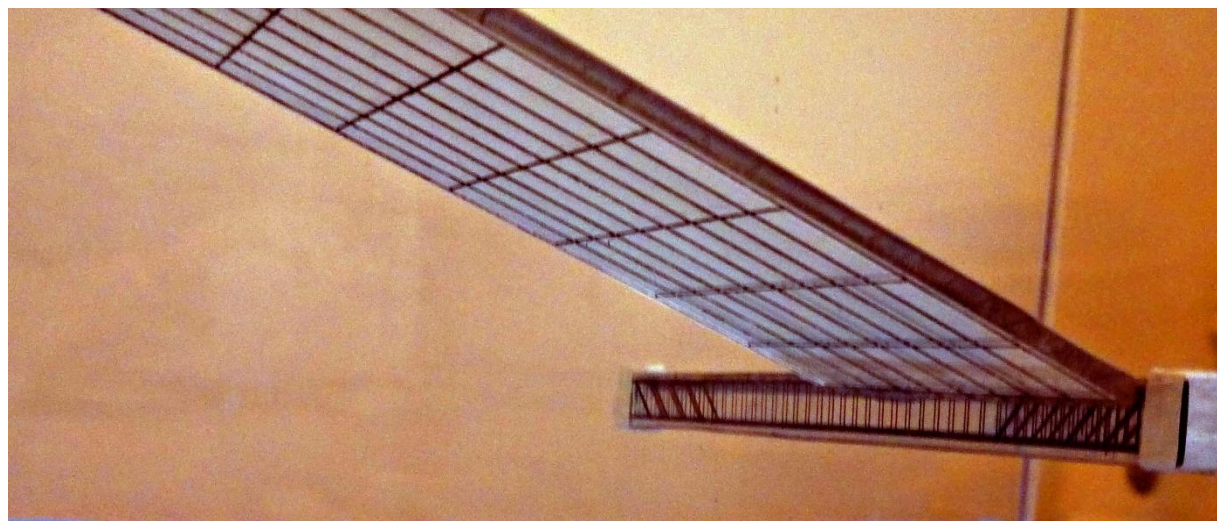
Figure 5: The model of the slab-beam stairs. A bottom reinforcement of the stair flight slab and the support beam
