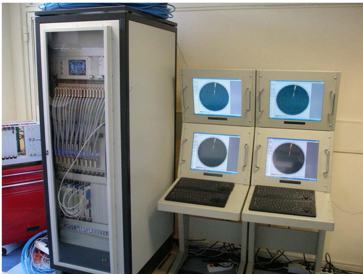
Fig.2. The Digital Signal Processing Unit and Operator Consoles of the modernized ASW sonar SQS-56 during the laboratory testing
