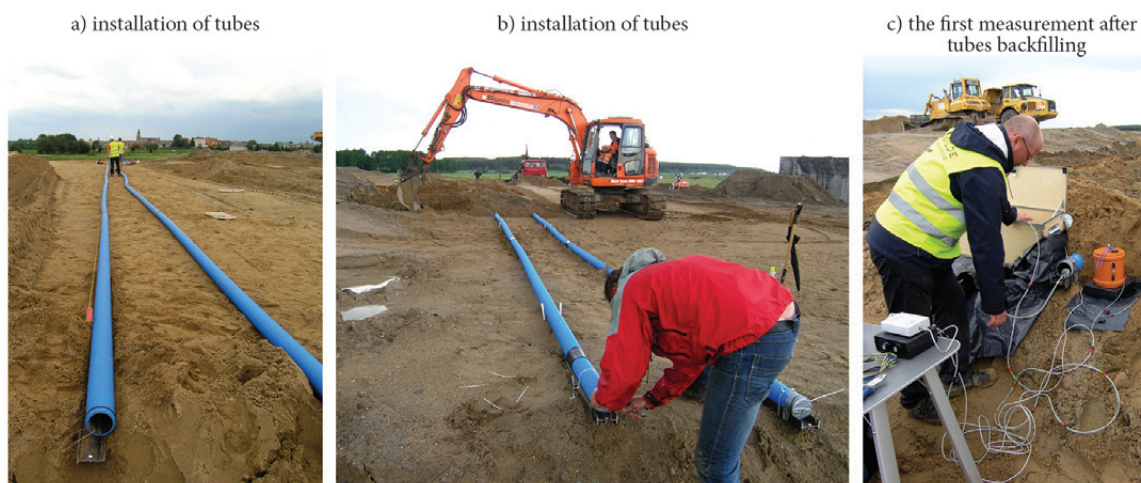
Fig. 8. Embankment settlement measurement by hydrostatic levelling
