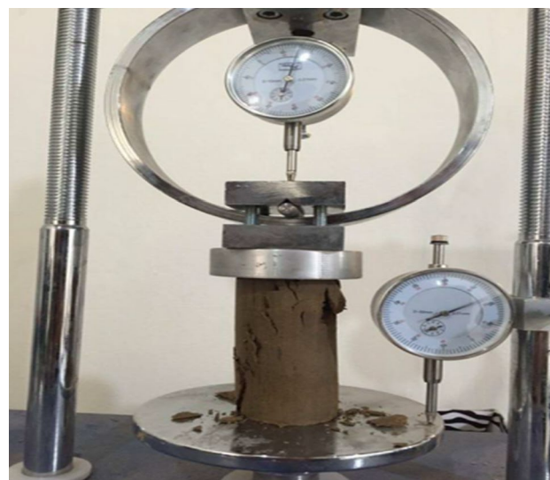
Figure 4. Specimen image after the UCS test.
