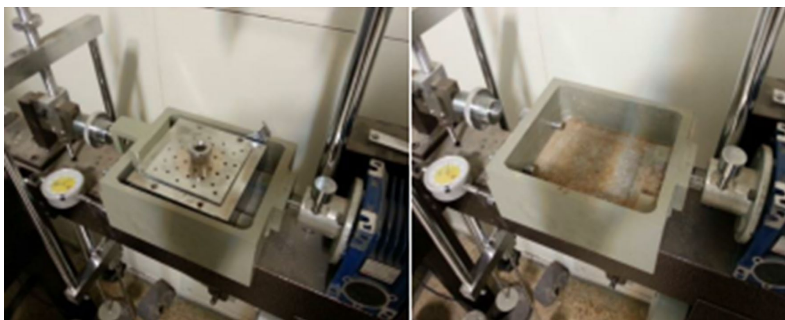
Figure 5. Direct shear test device used herein.
