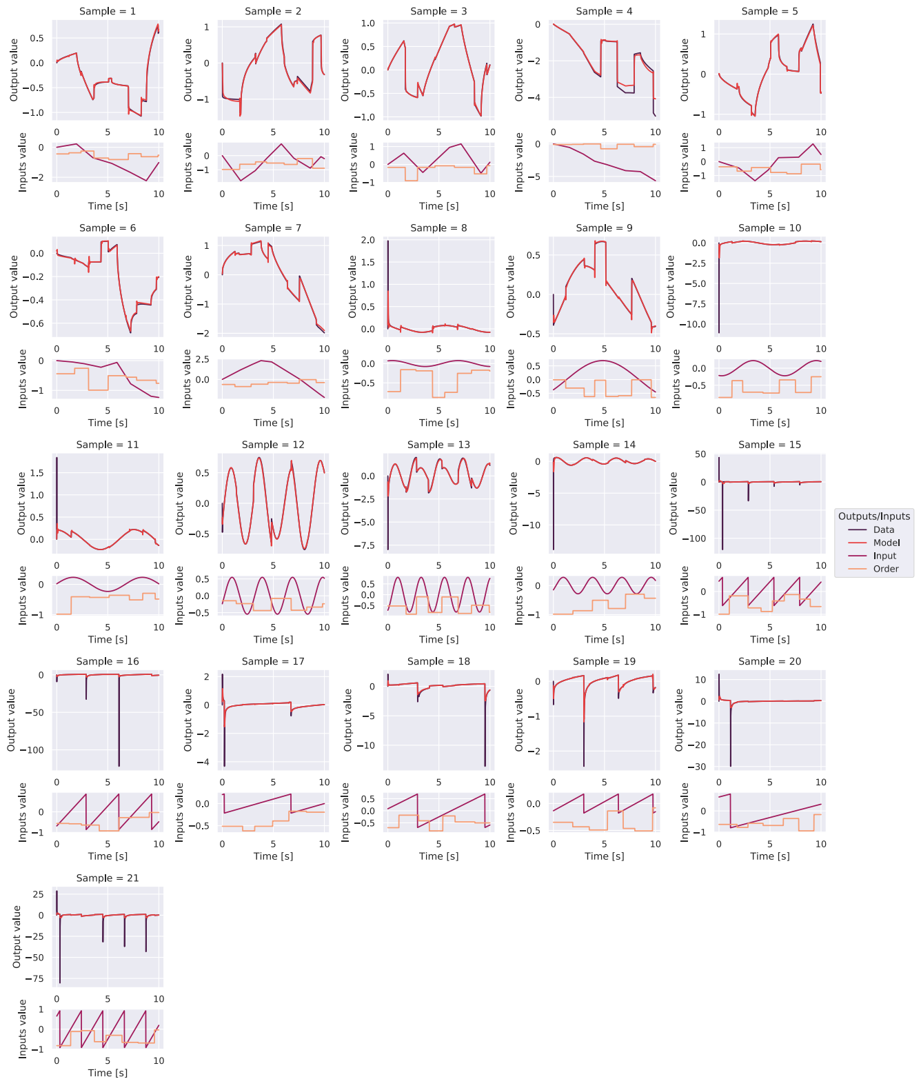
FIGURE 5. Responses to test signals for the best neural network for the differentiation operator. For each sample, the input signals are given in smaller plots.
