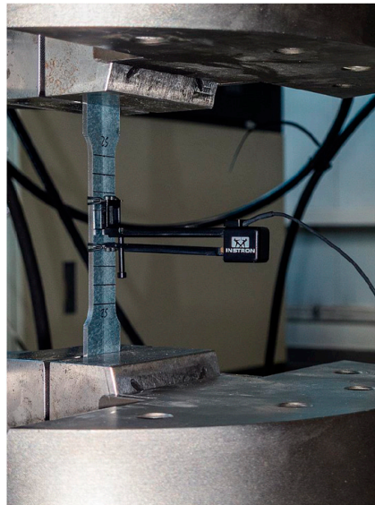
Figure 6. Material sample with an extensometer during testing.
