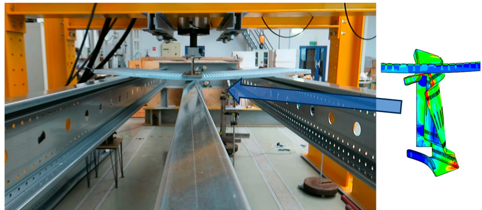
Figure 11. Loss of stability (buckling) of the central 6 m beam.
