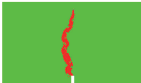
Fig. 20. Effect of aggregate stiffness on force-deflection curve and distribution of non-local strain measure close to beam notch: a) strong circular aggregate, b) weak circular aggregate (fine-grained concrete beam 80 \times 320 \text{ mm}^2 , l_c = 1.5 \text{ mm} , circular aggregate distribution 'c' of Fig. 2 with d_{50} = 4 \text{ mm} and d_{max} = 10 \text{ mm} , \rho = 60\% ).
