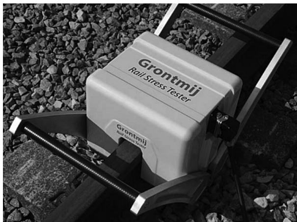
Rys. 7. Urządzenie Rail Stress Tester firmy Grontmij [31] Fig. 7. Measuring device Rail Stress Tester by Grontmij [31]
