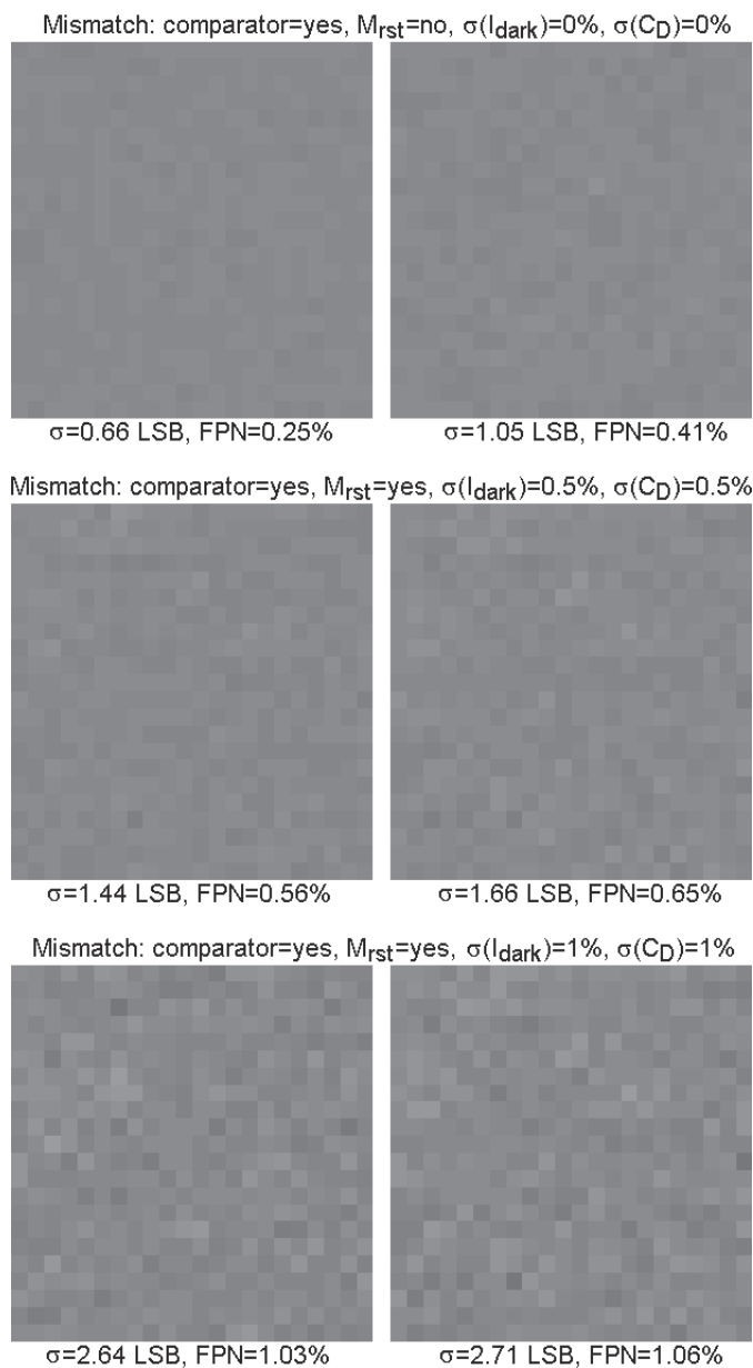
Fig. 7. Dark FPN noise in digital pixel matrices. Left column: pixels with complex comparators (Comparator I); right column: pixels with simplified comparators (Comparator II). Brightness and contrast of the images have been enhanced for the sake of better visualization
