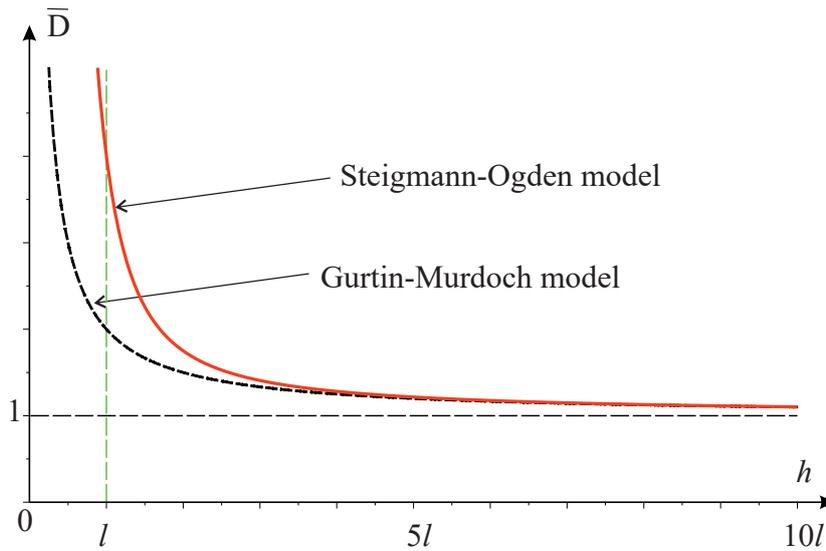
**Figure 2.** Dimensionless bending stiffness  $\bar{D} = D_{eff}/D$  vs. thickness  $h$  (solid red curve). The dashed blue curve corresponds to the Gurtin–Murdoch model; the horizontal dashed black line describes the classic bending stiffness. Finally, the vertical dashed green line marks the characteristic length  $l$  defined as  $l = (\lambda^S + 2\mu)h^2/D$ .
