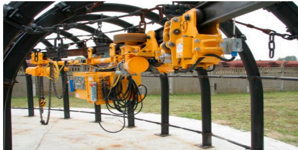
Figure 3. Operation of a suspended battery vehicle (PCA-1).
