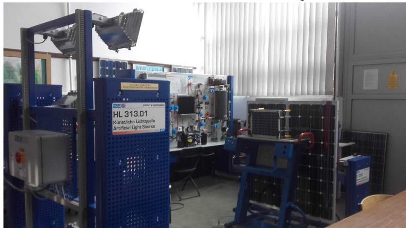
Fig. 3. Experimental stand for PV/PCM examination.
