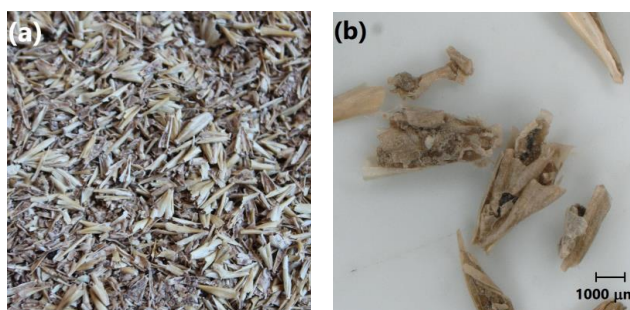
Figure 2. Macroscopic (a) and microscopic (b) appearance of applied brewers' spent grain (BSG) before extrusion grinding.
