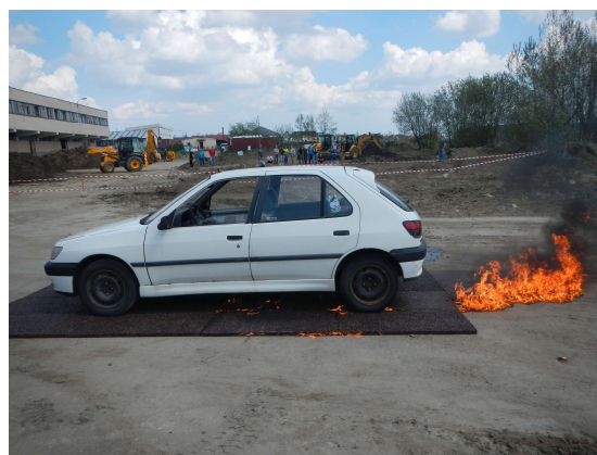
Fig. 10. Fuel fire on PERS (after 10 s).
