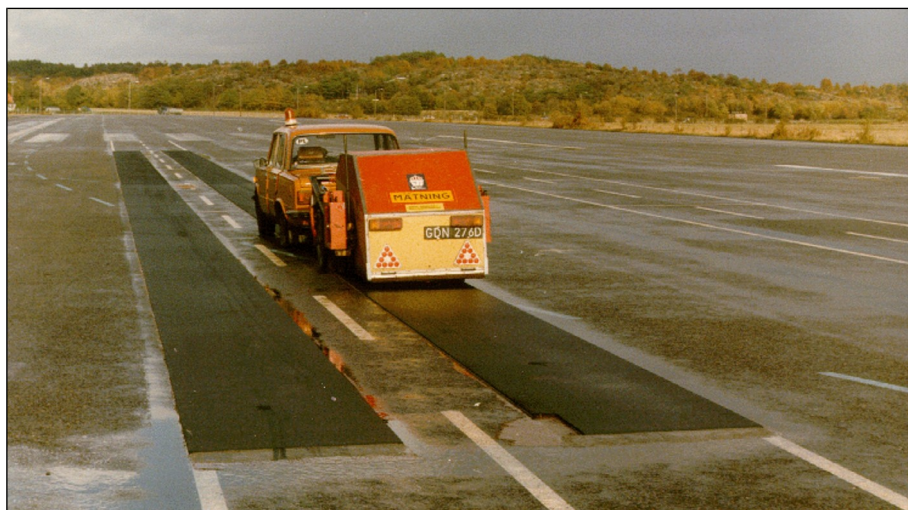
Figure 2: CPX measurements of poroelastic road pavement on Torslanda Airport by Tiresonic Mk. 1 trailer
