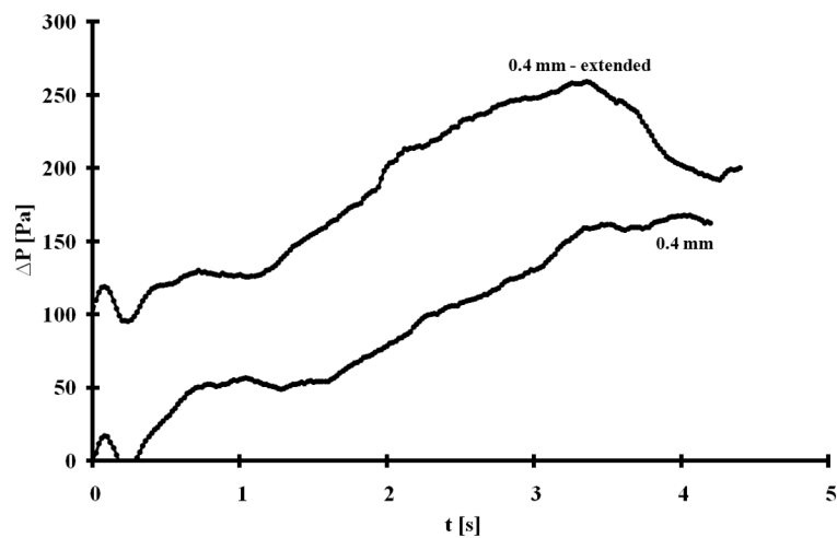
Figure 20: Comparison of local pressure drop as a function of a section filling time for basic and extended geometry and for average flowrate of 0.66 g/s.
