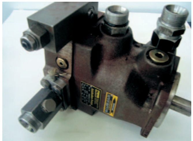
Fig. 3. Past-plate axial pump from Parker [21] company
