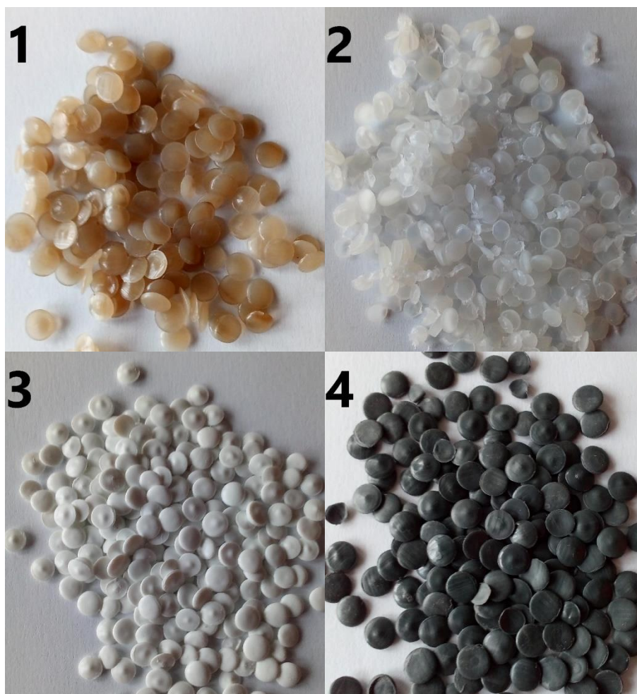
Fig. 1. The appearance of analyzed recycled LDPE streams.
