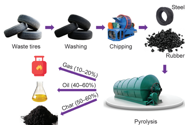
Figure 3. Waste tire pyrolysis process.
