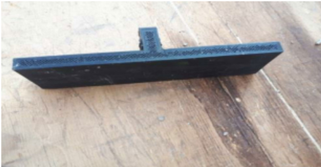
Fig. 3. Polymer plate anchors used in the present research.
