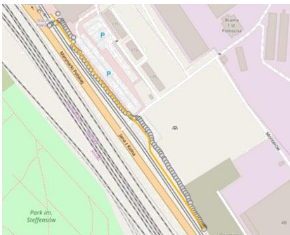
Fig. 11. Bicycle excursion along the straight line route with smartphone 2: yellow – real route, dot – measured route
