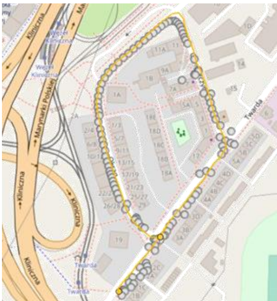
Fig. 5. Car excursion along the square-shaped route with smartphone 1: yellow – real route, dot – measured route
