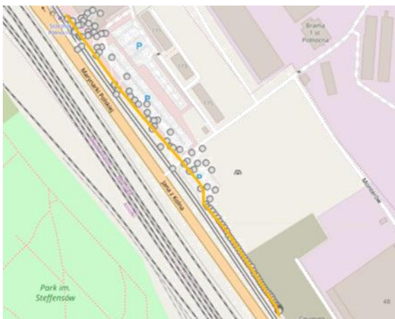
Fig. 9. Car excursion along the straight line route with smartphone 1: yellow – real route, dot – measured route
