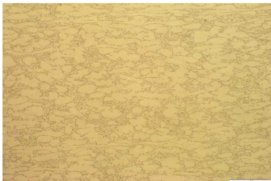
Fig. 3. Microstructure of the two ( \alpha + \beta ) phase Ti6Al4V alloy
