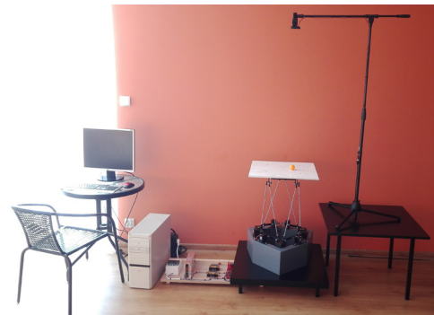
Fig. 3. A complete ball & plate control system research station
