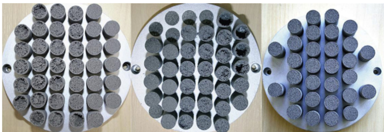
Figure 4. Porous samples made for permeability measurements [25].
