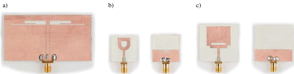
Fig. 4. Photographs of the fabricated prototypes of Antennas I through III optimized using the proposed algorithm: a) Antenna I (gain optimization); b) Antenna II; c) Antenna III.
