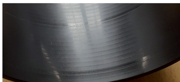
Fig. 6. Bearing surface after a series of tests in water lubrication
