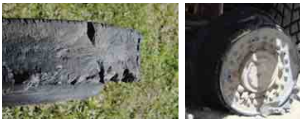
Fig. 2. Run Flat insert - wear and tear [photo: archives]
