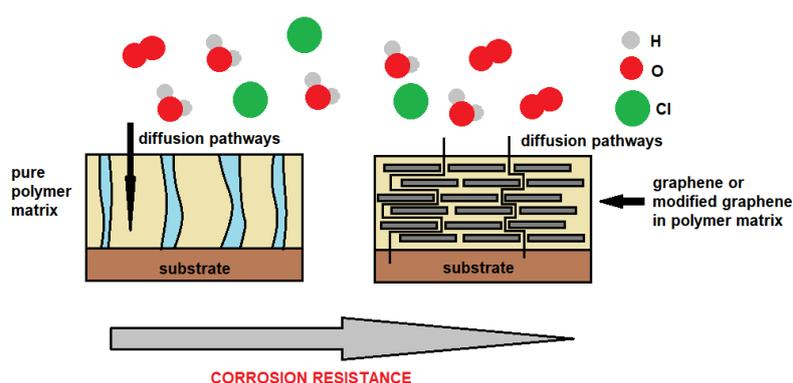
Figure 4. Mechanism protection of graphene polymer-based coatings.
