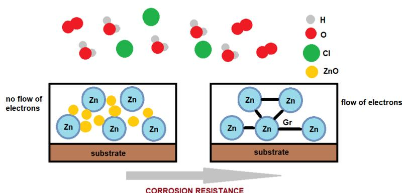
Figure 3. Mechanism protection of zinc-rich polymer coatings.
