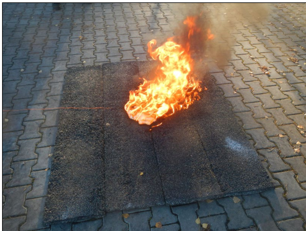
Figure 7. Fire of PERS material 180 seconds after ignition of 2.5 litre of gasoline - mostly cotton wool is burning
