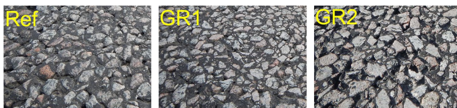
Figure 13. View on grinded test surfaces
