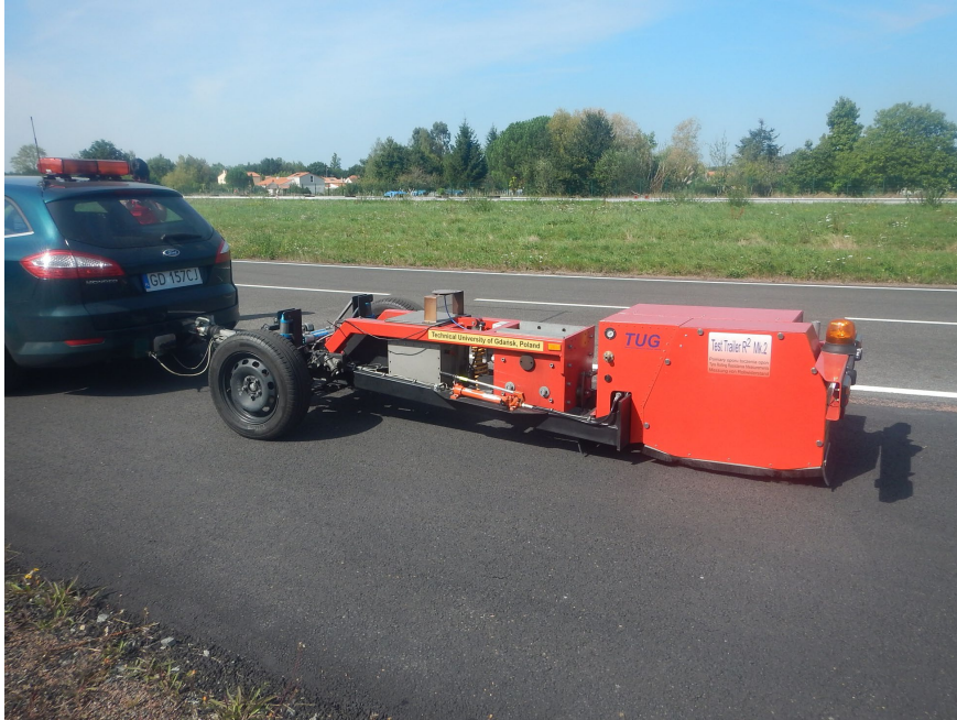
Figure 9. Rolling resistance test trailer R^2 Mk.2
