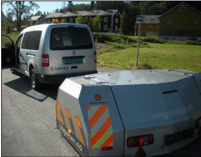
Figure 9. CPX test trailer used by SINTEF, Norway
