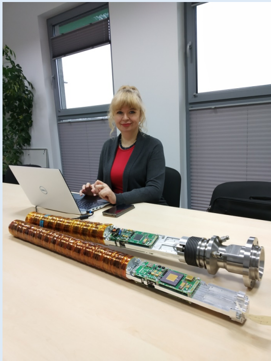
FIGURE 6 – High precision downhole monitoring system using high-temperature electronics developed by MMB Drives.
