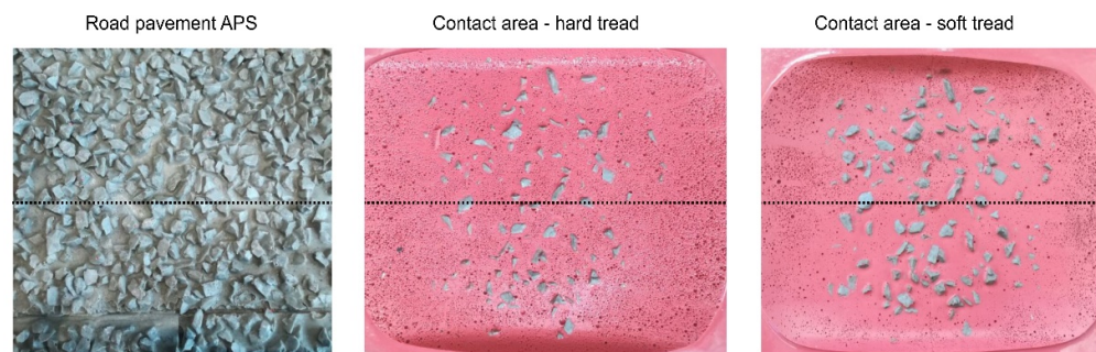
Figure 12. View of APS pavement and contact area of HARD and SOFT treads.
