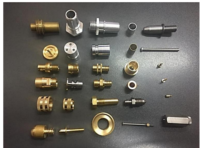
Fig. 1. Workpieces made on CNC turning centre
