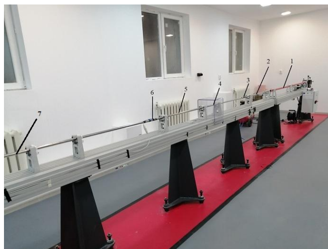
Fig. 1 Split Hopkinson-Kolsky pressure bar 1- Launching device, 2-Incident bar, 3-Strain gauges in the middle of IB, 4- Test piece, 5-Transmitted wave bar, 6- Strain gauges in the middle of TB, 7- motion suppression bar.
