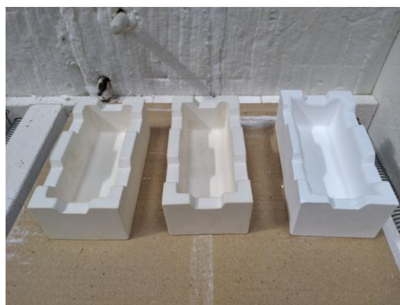
Fig. 3. High temperature synthesis of technical products with fixed thickness – refractory containers made of quartz glass ceramics, moulded in a gypsum mould with a silicone insert.
