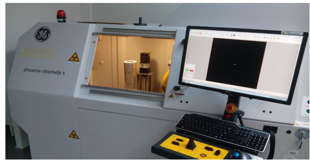
Fig. 1 General view of the GE phoenix vltomelx s240 CT equipment used for scanning selected granular materials (color figure online)
