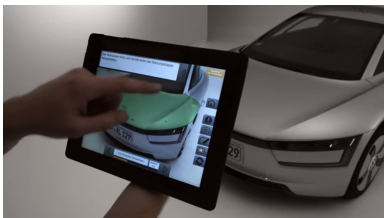
Figure 2.14: Guiding an auto mechanic with the MARTA application [133].
