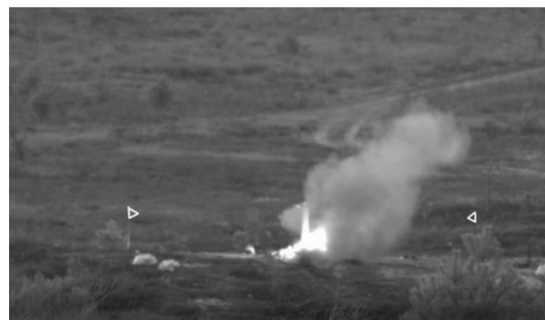
Fig. 7 Jet-fire after puncturing acetylene cylinder
