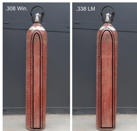
Fig. 4 Zones of efficient hit for the acetylene cylinders; solid line - efficient zone for FMJ, Match bullets and tracers, dotted line - efficient zone for AP bullets
