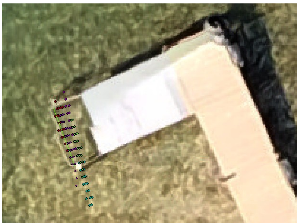
Figure 11. Photogrammetric and radar picture of a metal structure on a wooden jetty used for accuracy determination.
