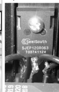
Fig. 7. The laboratory setup with proposed 50 kHz SiC-based DHB converter with 2 kW power planar transformer: circuit schematic (a); the overall view (b); investigated SiC MOSFET (c) and SiC JFET (d).
