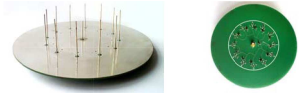
Fig. 3. Realized ESPAR antenna (top and bottom).
