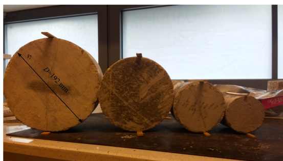
Fig. 3. The specimens with plywood strips scaled proportionally with specimens' diameter ( b/D = \text{const.} ) [22].
