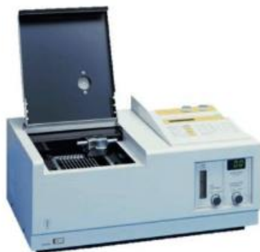
Fig. 2. TLC-FID analyzer (left) and the main part of the analyzer: quartz rods used for SARA tests (right) 25
