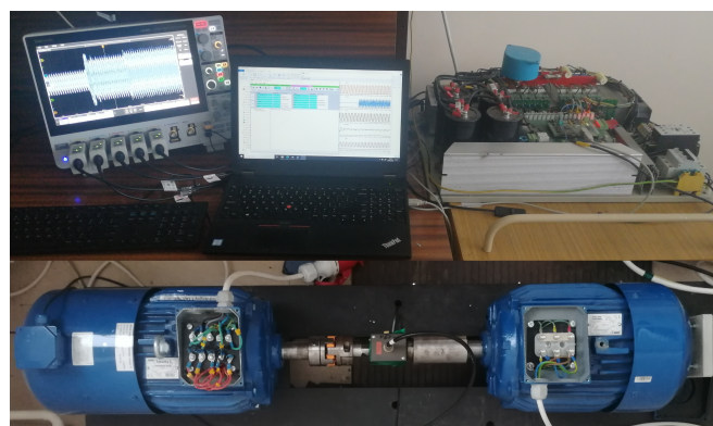
Fig. 12. Laboratory stand with 5-phases induction motor (left) and induction motor emulated the load (right).
